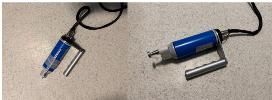
Fig. 1. The ^{57}\text{Co} source (left) and ^{137}\text{Cs} source (right) fixed to the B-RAD probe.
