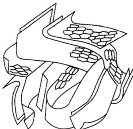
Figure 4.1 - Schematic representation of the microstructure of an activated carbon. Adapted from [2] .
