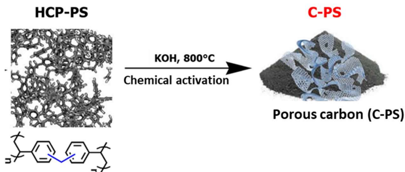
Figure 4.14 - Scheme of the preparation treatment HCP-PS with KOH, to obtain porous carbon (C-PS).
