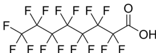
Figure 7.7- Molecular structure of Perfluorooctanoic Acid (PFOA).
