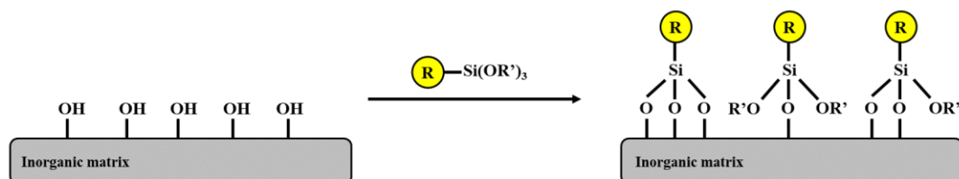
Figure 1.7. Grafting of specific ((R'O)_3SiR organosilanes, with R = organic functional group, onto the inorganic surface. [12]
