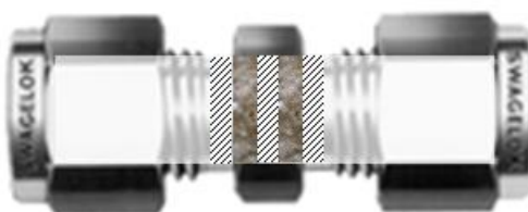
Figure 4.13. Adsorption column of ZLC instrument
