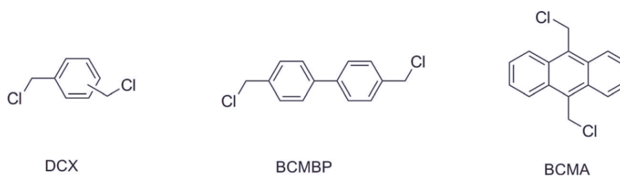
Figure 11. Example of monomers used for the synthesis of the HCP networks. Adapted from ref. 111
