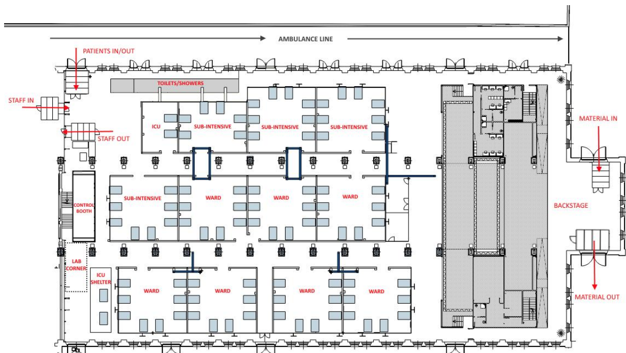
Figure 5.2 Red-zone layout of the OGR Temporary Hospital.
