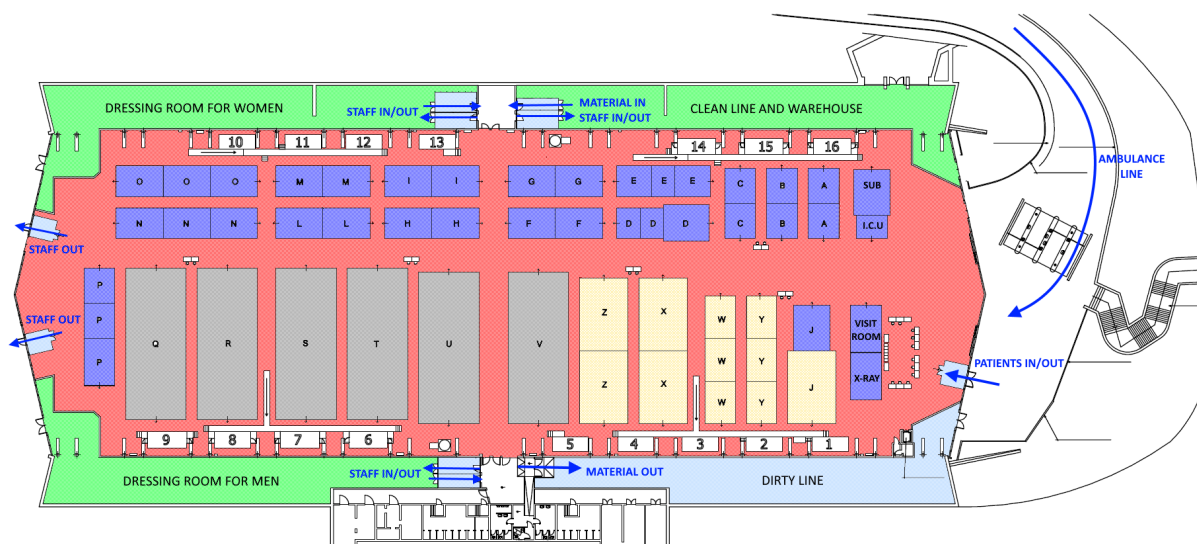
Figure 5.4 Layout of the Valentino Field Hospital. The areas dedicated to the personnel, such as the administrative desks, the canteen and the kitchen, the toilets and showers are not displayed in the figure since they are located outside of the underground parking.
