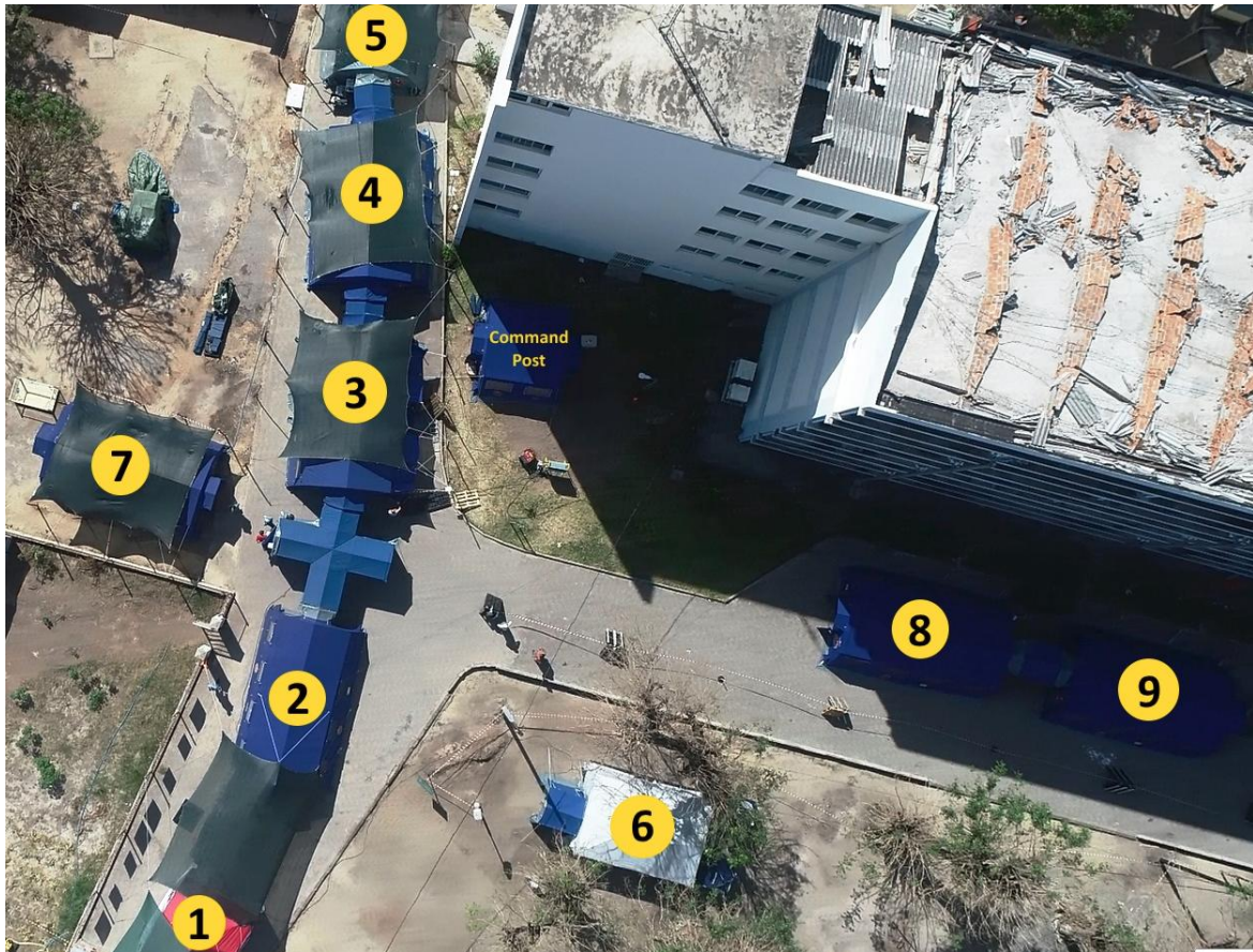
Figure 2.2 Deployed field hospital within the courtyard of the Central Hospital of Beira: (1) triage and registration, (2) emergency room (ER), (3) shock and critical care room with a gynecological corner, (4) post anesthesia care unit and sterilization room, (5) operating theatre (OT), (6) isolation room for suspected or confirmed infectious disease, (7) x-ray and laboratory, and (8)(9) inpatient wards.
