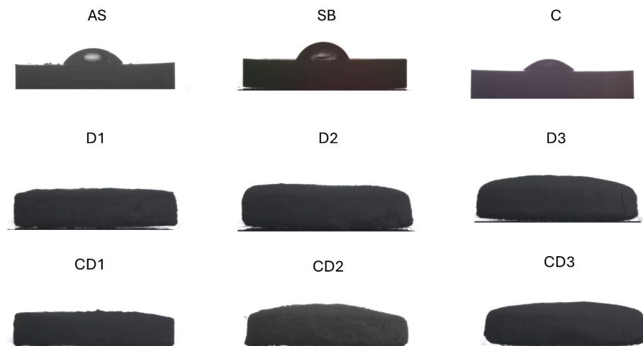
Fig. 9. Images of water droplets on the surfaces of the produced samples.
