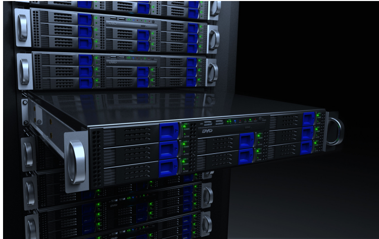
Figure 2.4: A server rack is a structure that is designed specifically to house technical equipment including routers, switches, hubs, and of course, servers.
