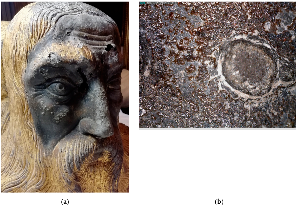
Figure 3. Globular alteration products: (a) photography of the face of Saint Venanzio; (b) details acquired by optical microscopy on the face of Saint Ruffino.
