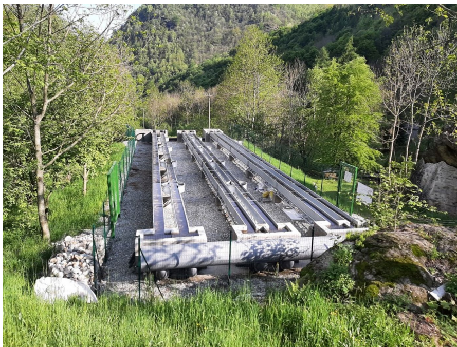
Fig. 1 Outdoor artificial flumes in Ostana (Italy) used in the experiment. Flume n.1 is on the right, while flume n.6 is on the left. Flumes are fed by the Po River via a water diversion located around 50m upstream
