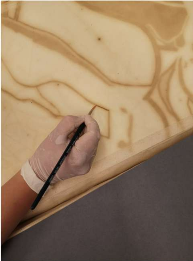
Figure 12: Application of a 3 % BTA solution by brush on brown discolouration on the verso of a map.
