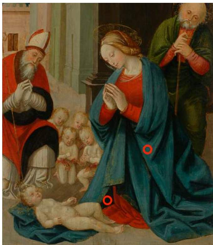
Figure 8. Measurement points (red circles) on the Virgin’s mantle in 483/D. FORS spectra acquired onto the light blue rope can be assigned to azurite while the dark inner part of the veil gives reflectance spectra of blackened azurite.
