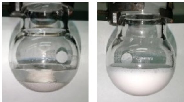
Fig. 1 Dispersing capabilities of TX-100 on chloride 1. Left: granules of derivative 1 in plain water. Right: chloride 1 in TX-100 10 wt% after 2 h stirring at r.t.
