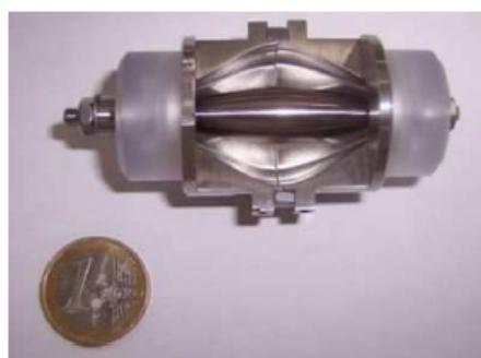
Figure 14: Real dimension of Orbital trap. Provided by Thermo Fisher Scientific.
